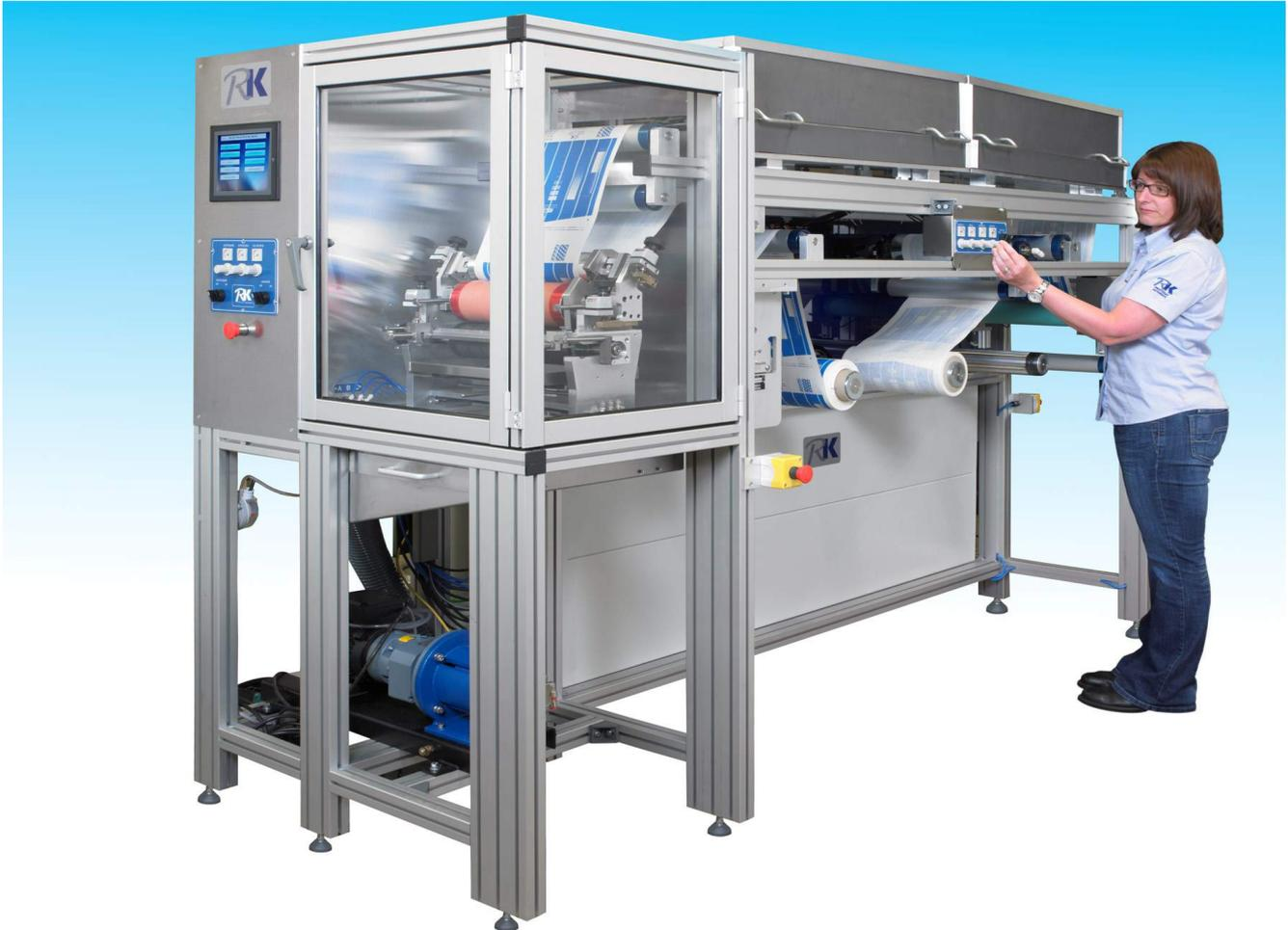
The VCML is designed to print, coat and laminate all types of flexible webs such as papers, films, and metallic foils on a reel-to-reel basis. With the ability to apply various coatings such as inks, paints, varnishes, adhesives both solvent and water based, by various application methods, this makes the VCML particularly useful for product development, quality control and small scale production for low volume of a specialised product.
