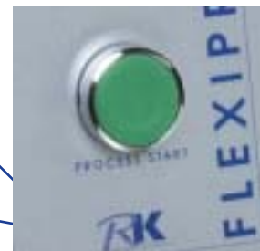
Dual start buttons for safety
